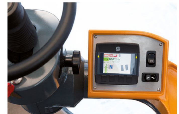
Control of the hydraulic pulling out of the batteries.
