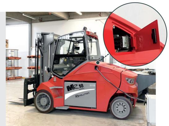
Batteries are recharged in direct mode, by means of the connector located in an easy-to-reach position and kept safe behind a handy hatch, as with electric cars.
