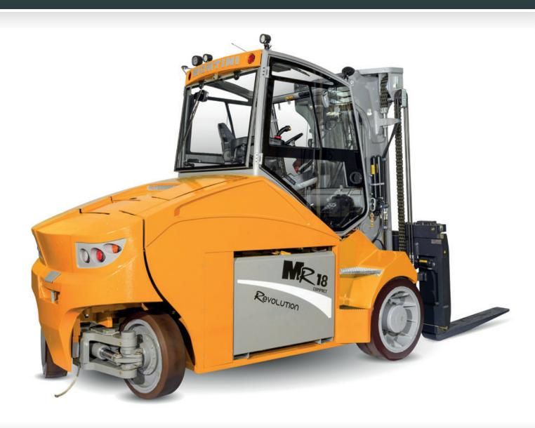
THE NEW 120V **COMPACT** FORKLIFT TRUCK WITH LOAD CAPACITY OF 18000 KG
