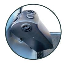
The **heater**, available as an optional extra, directly and quickly heats up the cab interior thanks to the hot air vents, thus making sure that the temperature inside the cab is always comfortable.
