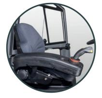
The driver's seat has been optimized for maximum ease with comfortable **seats** to meet the ergonomic needs of the operator.
