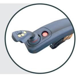
The simple to use and easily accessible hydraulic control with **fingertips** (mini-levers) is installed in an ergonomic and adjustable armrest.
