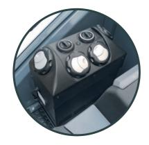
The **air conditioning unit**, available as an optional extra, is located in a handy position to the side of the seat. It creates a pleasant climate thanks to the various ventilation outlets.
