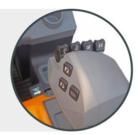
The **hydraulic control with pilot levers** (minijoysticks) makes driving the forklift truck easy and reliable.
