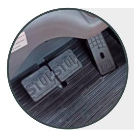
A large, spacious pedal board with a **single drive pedal** (with forward/reverse switch button on the provided hydraulic control armrest) combined with a large brake pedal.
